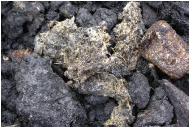
Figure 6. Insulating materials containing asbestos in soil.
