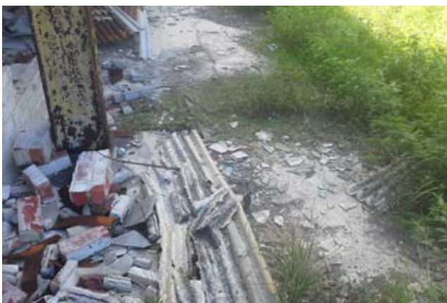
■ Figure 9. Other asbestos-containing products in soil.
