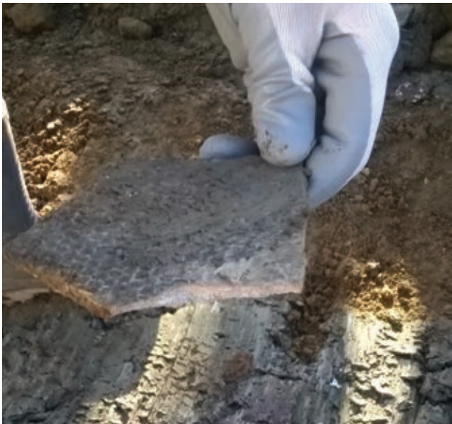
Figure 7. Asbestos-cement sheet and bonded ACM in soil.
