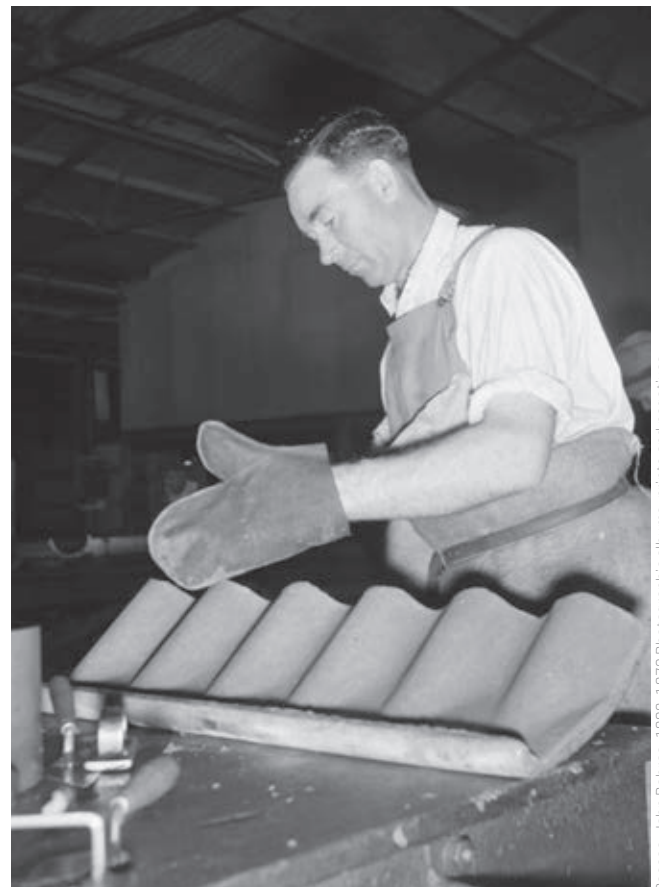
Figure 2. Manufacturing asbestos fibrolite [ca 1940s].
